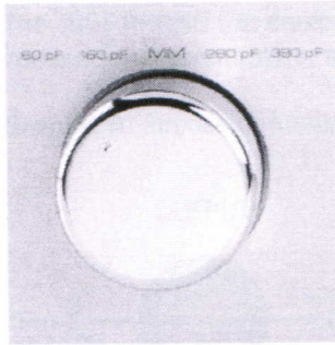
Graphic 5: Turning the MM rotary knob to select the input capacity
