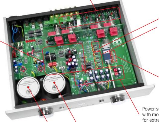
Balancing stage for unbalanced inputs with high precision ICs (TI OPA2107)
